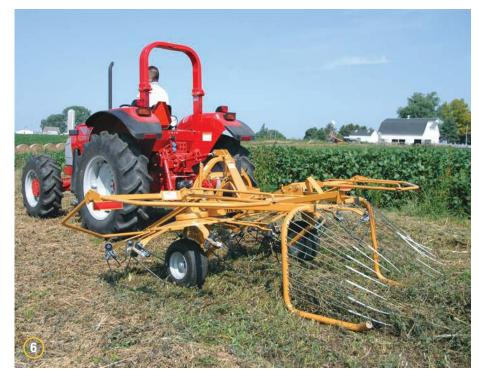
6 With new automatic field transport locks, you can engage and disengage the transport lock without leaving the tractor. The field transport locks will automatically lock when folding in and can be disengaged by pulling a rope from the tractor seat.
