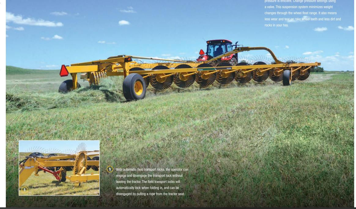
With a lift/suspension cylinder on each wheel and the nitrogen-charged accumulator, adjusting rake wheel pressure is efficient. Change pressure settings using
