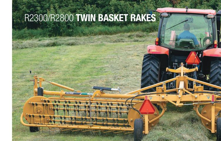
(1) Change rake/windrow widths hydraulically to help maximize raking efficiency and custom-shape the windrows to your baler pickup. Optional basket speed control (only available on the R2300) also allows you to adjust the raking action of the baskets for different crops and conditions.
