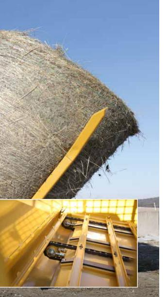
2 The slat and chain bale rotation design feeds bales consistently into the rotor — reducing the need to reverse rotation. Heavy-duty sprockets and chains allow misshaped bales to be processed smoothly. Split shafts let you perform maintenance without removing the entire bed.
