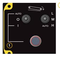
1 The automatic bale feed system helps optimize productivity and provides smooth material feeding through automatic slow down or speed up to maintain a consistent operating PTO and rotor rpm. All this makes it easier for the operator to manage the feeding system.
