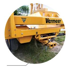
The hitch is located on the loading side of the machine for ease of access to the tongue. This allows operators to pull the machine away from the line of bales without requiring a power drive on the bale wrapper.
