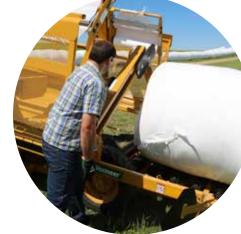
4 Optional spring-assisted final bale push-off feature smoothly ejects the last bale from the wrapper.
