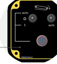
4 Hydraulic controls provide operators the ability to choose how the spout is angled and how the crop is distributed.
