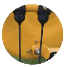
6 Six bar baskets on the R2300 (seven bar baskets on the R2800) mean maximized sweeping action, especially in high-volume conditions. Rubber-mounted tines can help reduce maintenance and service time.
