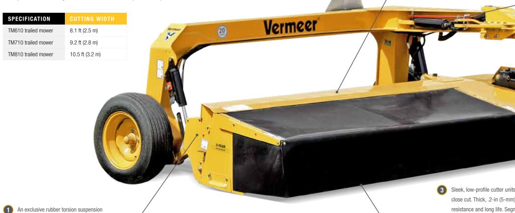
4 A side-pull rotary disc mower design with hydraulic swing cylinder makes transport convenient from field to field.
