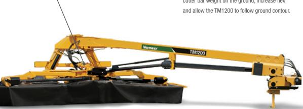
3 The TM1200 quickly folds down to 8.5 ft (2.6 m) to efficiently maneuver though gates when traveling from field to field, while the 2-point hookup accommodates both category II and III N hitches.
